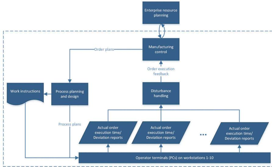
Figure 2. Functional description of the TDM IT system.
