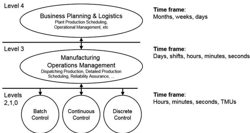
Figure 1. A functional hierarchy model of a manufacturing enterprise, adapted from ISA95 (2013).
