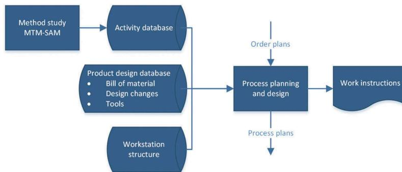
Figure 3. The elements of process planning and design.
